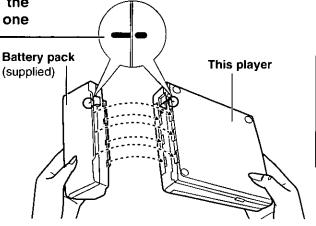
2 Slide the battery pack in the direction indicated by the arrow until the release button clicks.
